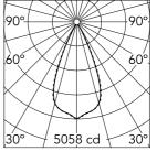
Luminous flux luminaire 2666 lm (EXTREME CUT OFF)
