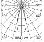
Luminous flux luminaire 2836 lm (EXTREME CUT OFF)
