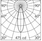
Luminous flux luminaire 157 lm
