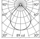
Luminous flux luminaire 193 lm
