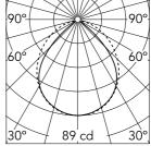
Luminous flux luminaire 193 lm
