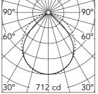
Luminous flux luminaire 1543 lm
