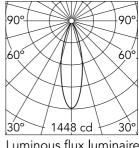
Luminous flux luminaire 417 lm (EXTREME CUT OFF)
