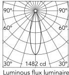
Luminous flux luminaire 550 lm (EXTREME CUT OFF)
