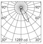
Luminous flux luminaire 718 lm (EXTREME CUT OFF)
