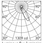
Luminous flux luminaire 682 lm (EXTREME CUT OFF)
