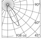
Luminous flux luminaire 620 lm (EXTREME CUT OFF)
