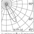
Luminous flux luminaire 806 lm (EXTREME CUT OFF)
