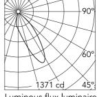
Luminous flux luminaire 861 lm (EXTREME CUT OFF)
