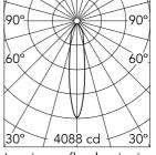
Luminous flux luminaire 955 lm (EXTREME CUT OFF)
