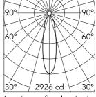
Luminous flux luminaire 903 lm (EXTREME CUT OFF)
