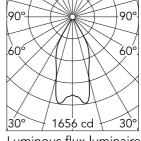
Luminous flux luminaire 960 lm (EXTREME CUT OFF)
