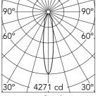
Luminous flux luminaire 1069 lm (EXTREME CUT OFF)
