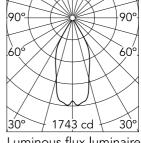
Luminous flux luminaire 996 lm (EXTREME CUT OFF)
