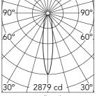
Luminous flux luminaire 696 lm (EXTREME CUT OFF)
