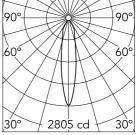
Luminous flux luminaire 740 lm (EXTREME CUT OFF)
