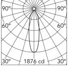
Luminous flux luminaire 641 lm (EXTREME CUT OFF)
