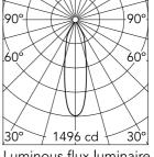
Luminous flux luminaire 495 lm (EXTREME CUT OFF)
