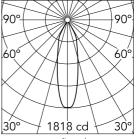
Luminous flux luminaire 630 lm (EXTREME CUT OFF)
