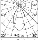
30° 943 cd 30° 5 Luminous flux luminaire 608 lm (EXTREME CUT OFF)
