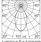
Luminous flux luminaire 596 lm (EXTREME CUT OFF)
