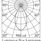
Luminous flux luminaire 620 lm (EXTREME CUT OFF)
