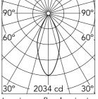
Luminous flux luminaire 977 lm (EXTREME CUT OFF)
