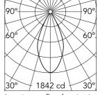
Luminous flux luminaire 1109 lm (EXTREME CUT OFF)
