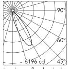
Luminous flux luminaire 2151 lm (EXTREME CUT OFF)
