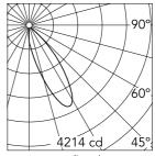
Luminous flux luminaire 1898 lm (EXTREME CUT OFF)
