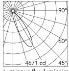
Luminous flux luminaire 1621 lm (EXTREME CUT OFF)
