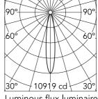
Luminous flux luminaire 1685 lm (EXTREME CUT OFF)
