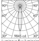
Luminous flux luminaire 1421 lm (EXTREME CUT OFF)
