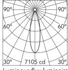
Luminous flux luminaire 1825 lm (EXTREME CUT OFF)
