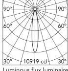
Luminous flux luminaire 1685 lm (EXTREME CUT OFF)
