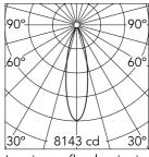
Luminous flux luminaire 2026 lm (EXTREME CUT OFF)
