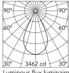
Luminous flux luminaire 2326 lm (EXTREME CUT OFF)
