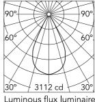
Luminous flux luminaire 2077 lm (EXTREME CUT OFF)
