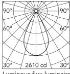
Luminous flux luminaire 1753 lm (EXTREME CUT OFF)
