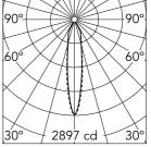
Luminous flux luminaire 762 lm (EXTREME CUT OFF)
