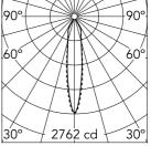
Luminous flux luminaire 771 lm (EXTREME CUT OFF)
