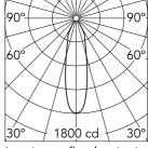
Luminous flux luminaire 639 lm (EXTREME CUT OFF)
