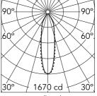
Luminous flux luminaire 640 lm (EXTREME CUT OFF)
