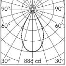
Luminous flux luminaire 666 lm (EXTREME CUT OFF)
