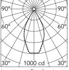
Luminous flux luminaire 685 lm (EXTREME CUT OFF)
