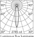
Luminous flux luminaire 732 lm (EXTREME CUT OFF)
