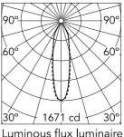
Luminous flux luminaire 582 lm (EXTREME CUT OFF)
