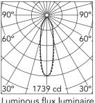
Luminous flux luminaire 624 lm (EXTREME CUT OFF)
