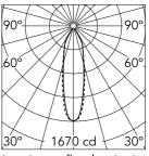
Luminous flux luminaire 640 lm (EXTREME CUT OFF)
