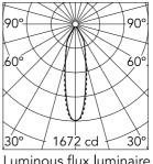
Luminous flux luminaire 600 lm (EXTREME CUT OFF)
